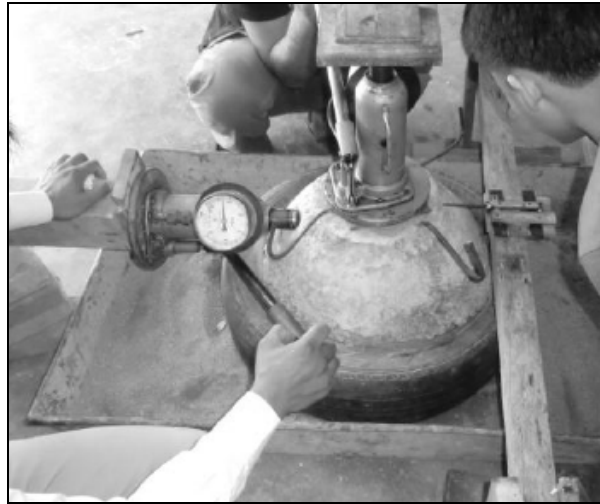
Figure 3. Tire-base-foot on sand (by Saevfors, 2010)
