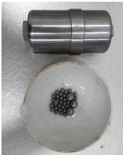
Fig 8 Tube and Balls for Fly Ash Milling Process
